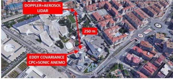
Figure 1. Experimental set up for the eddy covariance and remotes sensing setups at the urban area of Granada.
