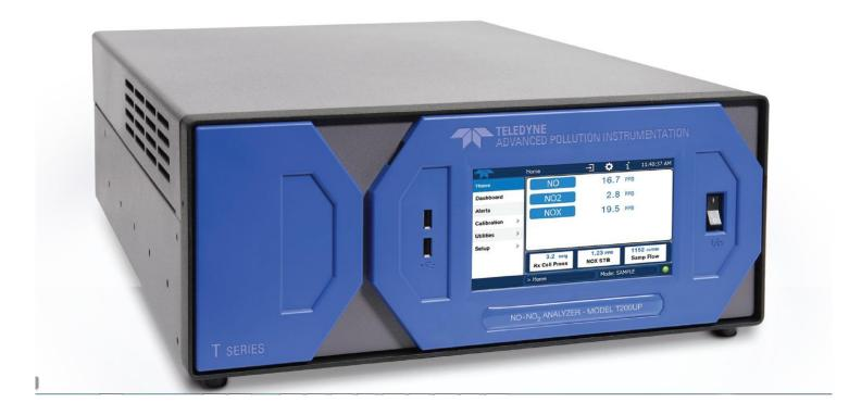
Transfer standard HORIBA Zero/span, linearity, checking efficiency by GPT (twice a year) Analyzer T200UP check (and adjust) the analyzer in four points every 23 h Dilution unit + Zero Air source + high Calibrator CMK concentration cylinder Zero/span
